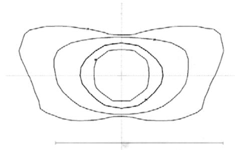
*GammaPlan solution for 201 beams of photons targeted at the centre of a spherical water phantom*
