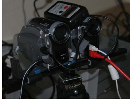
Figure 3: Sony camcorders ready for stereoscopic recording; including, fixed tripod mount, synchronisation LANC controller (black), USB web-streaming (white), high-speed tape download through fire-wire (red) and screw-fixable polarisation filters.
