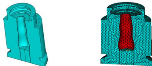
Figure 3: Finite Element Model of a Glass Mould.
