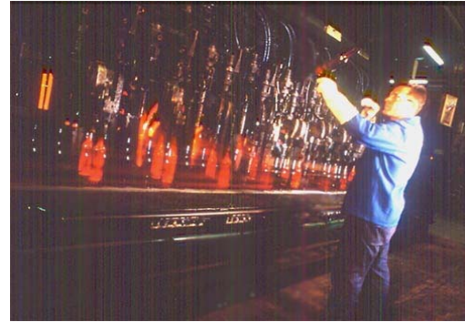
Figure 2: The Press-Blow Container Forming Process.
