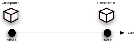
Figure 2: Checkpoints save the state of the simulation and are represented as cubes of data.
