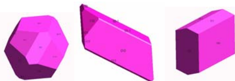
Figure 4 Left to right; predicted morphologies (Wulff plots) for piracetam forms I, II and III.
